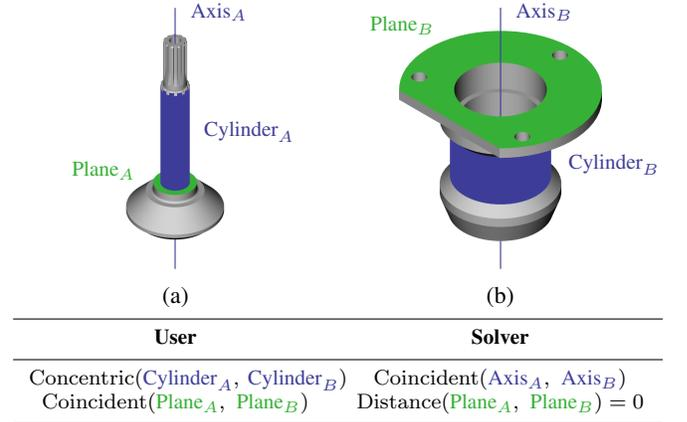
Fig. 6: Geometric constraints for the assembly of two workpieces
