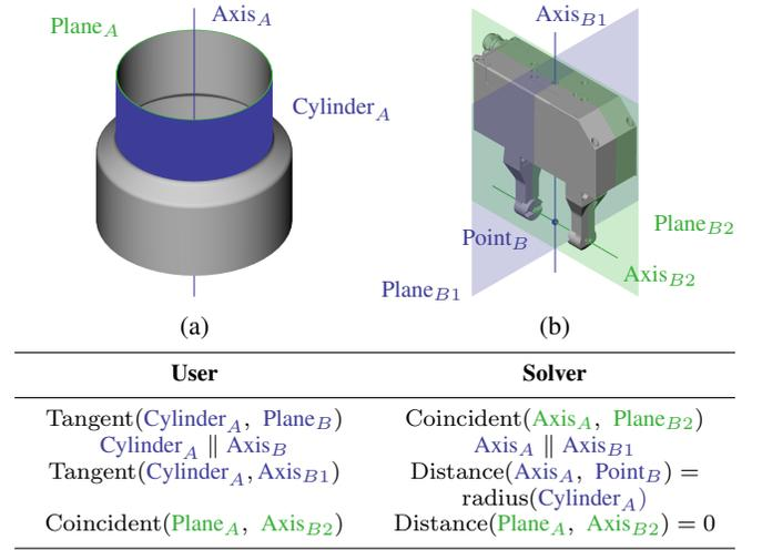
Fig. 5: Geometric constraints for grasping a cylindrical object at its rim
