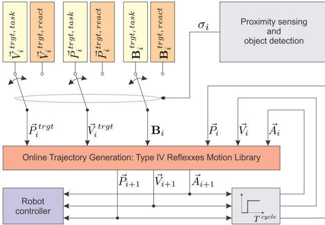
Fig. 7. Overview of one of the simplest possible robot motion generation architectures. The two sets of motion parameters *task* and *react* can be changed from one control cycle to another using the switching signal  $\sigma_i$ . The online trajectory generation algorithms [16] of the Reflexes Motion Library [17] let robots react to the input signals from the proximity sensor within the same control cycle they occur.
