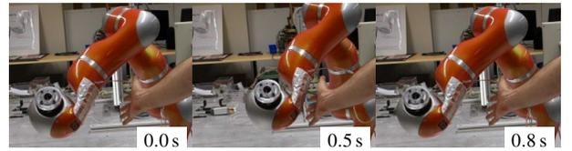
Fig. 8. A robot arm reacts instantaneously to the measurement data of the presented capacitive sensor. Capacitive sensing allows the robot to avoid collision with a human hand, maintaining a minimum distance of  $\approx 50$  mm.
