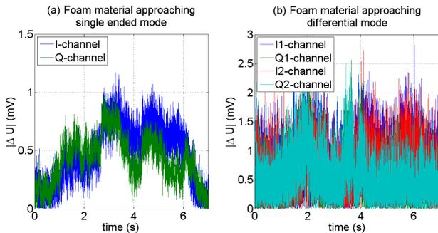
Fig. 15. Sensor signals for a foam material approaching to about 5 mm and leaving the sensor surface. Since the foam's electric susceptibility  $\chi$  is very low and it is of small volume/density it has only little influence on the electric field. Thus, it cannot reliably be detected by the measurement system.
