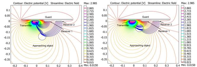
Fig. 3. A descriptive example on how an approaching object deforms the electric field.
