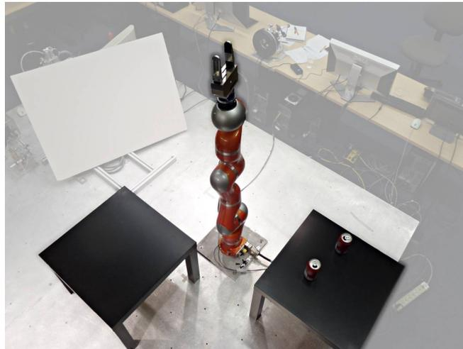
Fig. 1. In the FORCE SENSING scenario, a compliant robot manipulator can sense if beverage containers are filled by weighing them, and holding them upright while moving to prevent spilling, unless they are known to be completely empty or not opened.
